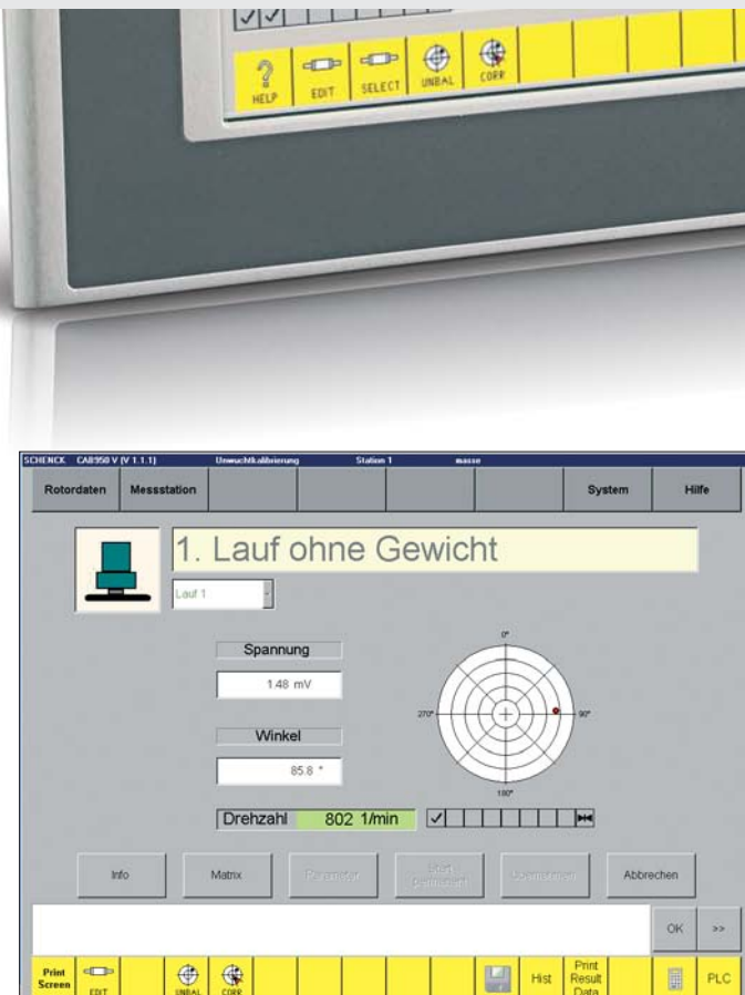
Calibration procedure of a vertical balancing machine
