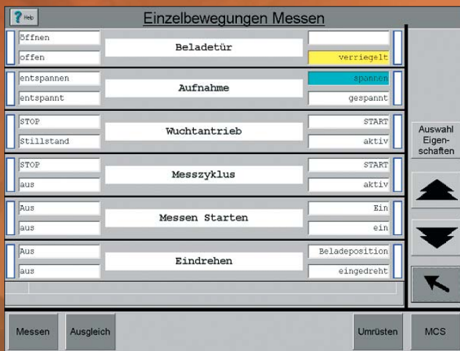
Individual movement with status display are visualised in the Siemens-Simatic ProTool / ProAgent-environment
